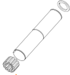
Cooling shroud A304 with bands A321 Motor centring ring A304 Pump centring ring SBR/NBR rubber with cutouts for motor cable (s)
