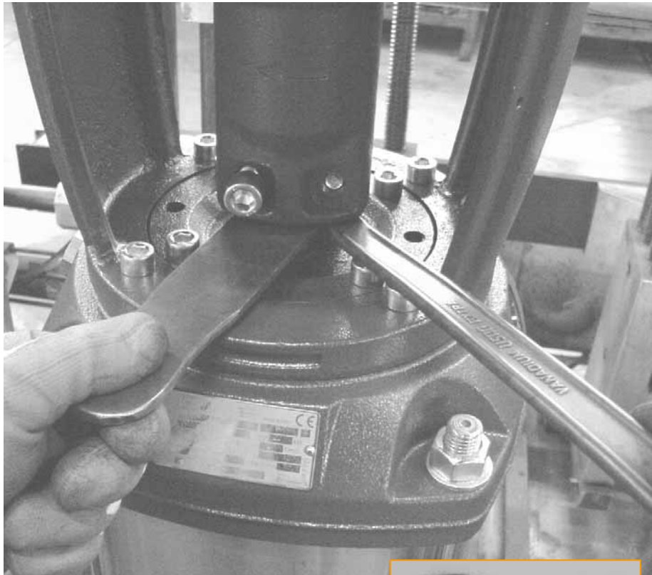
Coupling positioning – 5mm spacer →
