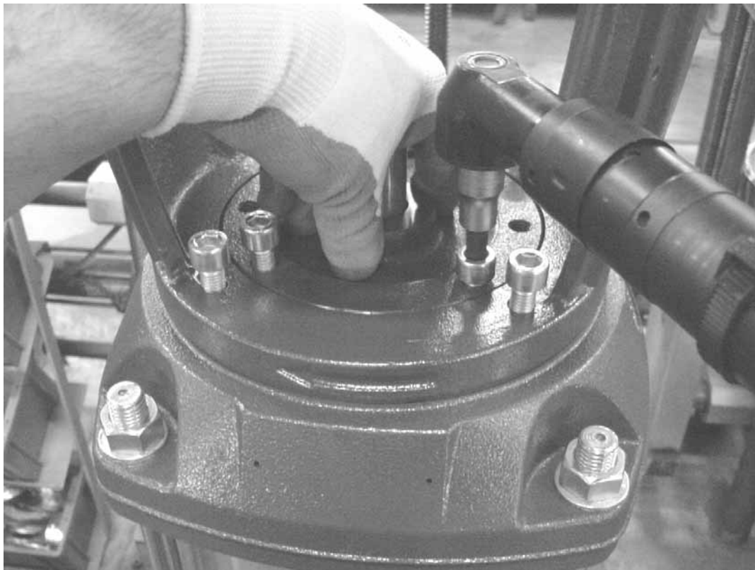
Seal housing disc installation Cross-tightening required.
